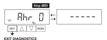
**Step 4BD** – Battery Pack Charge History. Displays the measure mAhrchargeofthebatterypackoverthepast63days. REGEN in the second display indicates that a regeneration occurred on that day. Press NEXT to exit Battery Diagnostics. Press REGEN to return to previous step.
