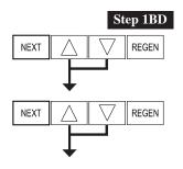
**Step 1BD** - Press  $\[ ]$  and  $\[ ]$  simultaneously for 5 seconds and release. Press  $\[ ]$  and  $\[ ]$  simultaneously for 5 seconds and release. If screen in Step 2BD does not appear the lock on the valve is activated. To unlock press  $\[ ]$ , NEXT,  $\[ ]$ , REGEN in sequence, then press  $\[ ]$  and  $\[ ]$  simultaneously for 5 seconds (twice) and release.
