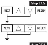
**Step 1CS** – Press NEXT and [] simultaneously for 5 seconds and release. Press NEXT and [] simultaneouslyfor5secondsandrelease. If the screen in Step 2CS does not appear, the lock on the valve is activated. Tourlock, press [], NEXT, [] and REGEN in sequence, then press NEXT and [] simultaneously for 5 seconds and release. Press NEXT and [] simultaneously for 5 seconds and release.
