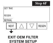
**Step 6F** – Set Regeneration Time Options using [] or []. NOTE: This step will not appear if Step 5F is set to oFF.
