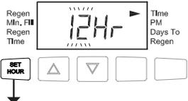
**STEP6SS** – Timekeeping format – only viewed when DC power supply is used. Use ▲ or ▼ to select 12 for 12 hour AM/PM format or 24 for 24 hour format.
