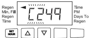
Typically a system is set to regenerate at a time of low water usage. An example of a time with low water usage is when a household is asleep. If there is a demand for water when the system is regenerating, untreated water will be used.
